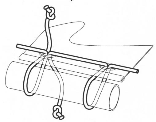
Canopy Lacing and Knotting: Lace only one grommet at the time pulling all cord thru before lacing the next grommet.
